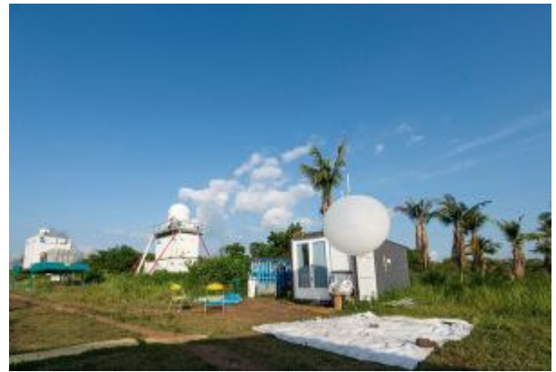
Using meteorological balloons and the atmospheric observation system „KITcube“, the climate researchers collected a variety of relevant meteorological data (photo: Sébastien Chastanet)
